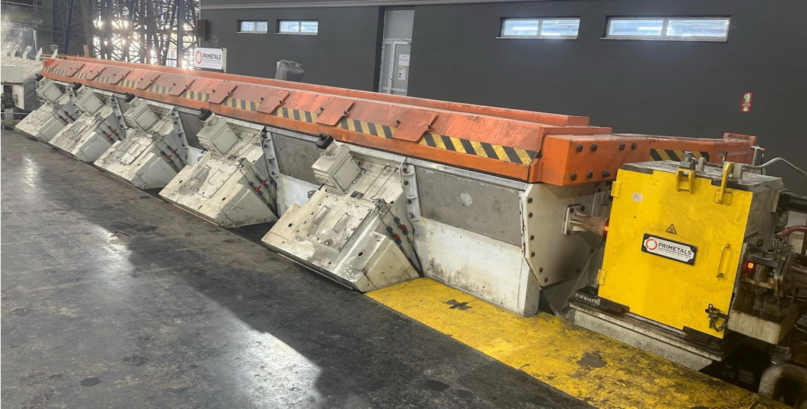
10-stand next-generation Morgan No-Twist mill from Primetals Technologies.
